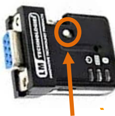
Ensure the slide switch on the Bluetooth transmitter is in the DCE position.
