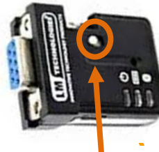
Ensure the slide switch on the Bluetooth transmitter is in the DCE position.
