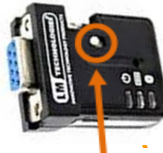
Ensure the slide switch on the Bluetooth adapter is in the DCE position.
